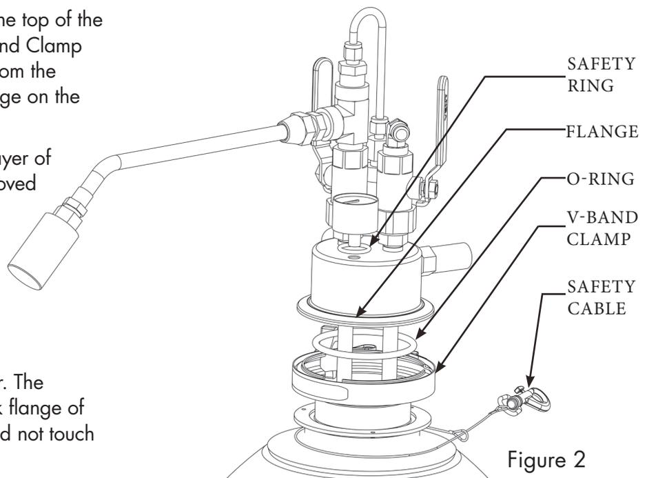
of the hose. If liquid nitrogen is trapped between the valves of the liquid cylinder and the LWD, it has no escape path as it warms and expands. The resulting pressure can cause the hose to rupture and may cause personal injury. The current model LWD is equipped with a pressure relief valve. Previous versions of the LWD must be used with a transfer hose equipped with a pressure relief valve.
