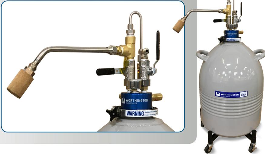
The Liquid Withdrawal Device (LWD) provides convenient pressure transfers of liquid nitrogen from LD25, LD35 and LD50 Dewars. The device clamps directly to the special neck flange that is found under the plastic trim collar around the neck of these containers.
